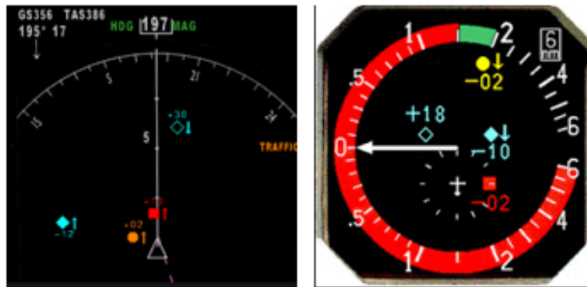
Figure 4: TA and RA Displays: The left display is the TA display and the right is the RA display [14].
